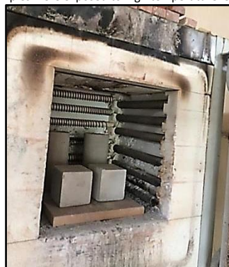
Figure 3. Foamcrete samples were exposed to high temperature. Source: Self-elaboration.
