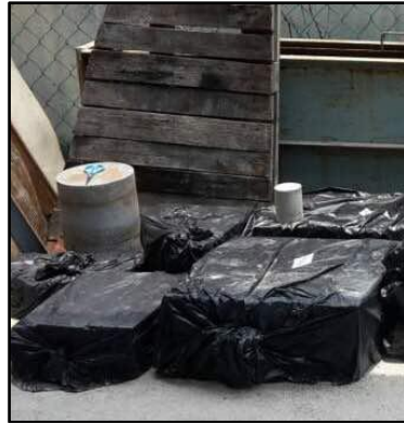
Figure 2. Lightweight foamcrete specimens were properly sealed cured with plastic sheets (PSC). Source: Self-elaboration.
