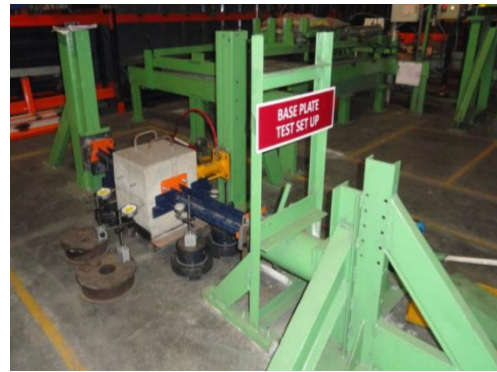
(c) Cross sectional view of the experimental setup as per BS EN 15512-2009
