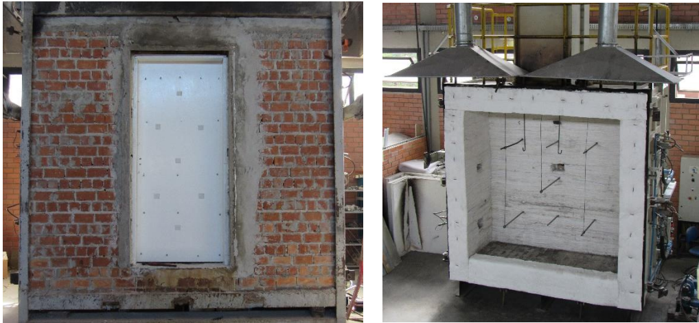
Figure 2. Sample assembled and vertical test furnace. Source: elaborated by the authors.
