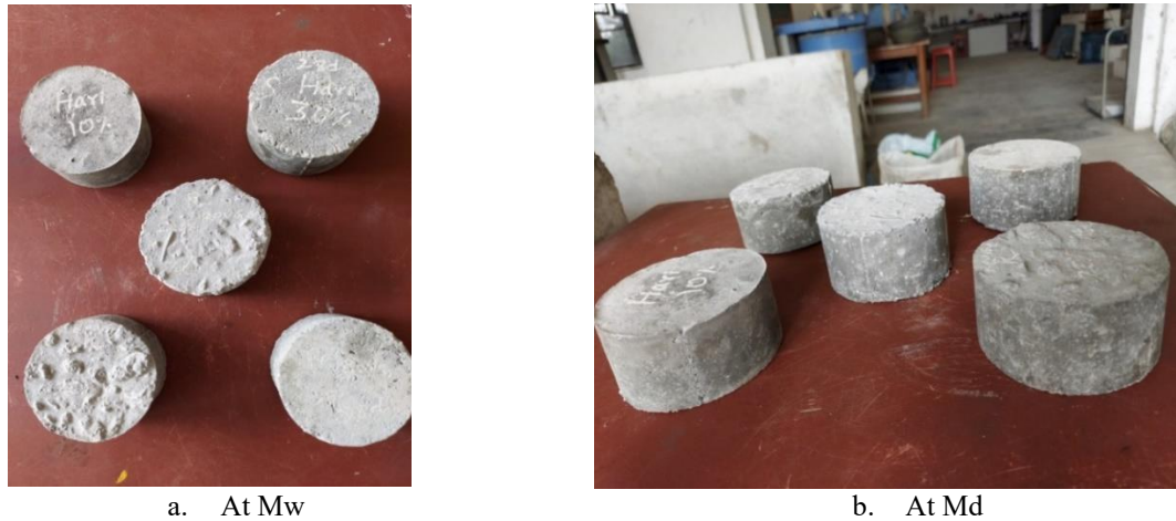
Figure 7. Test specimen for water absorption.
