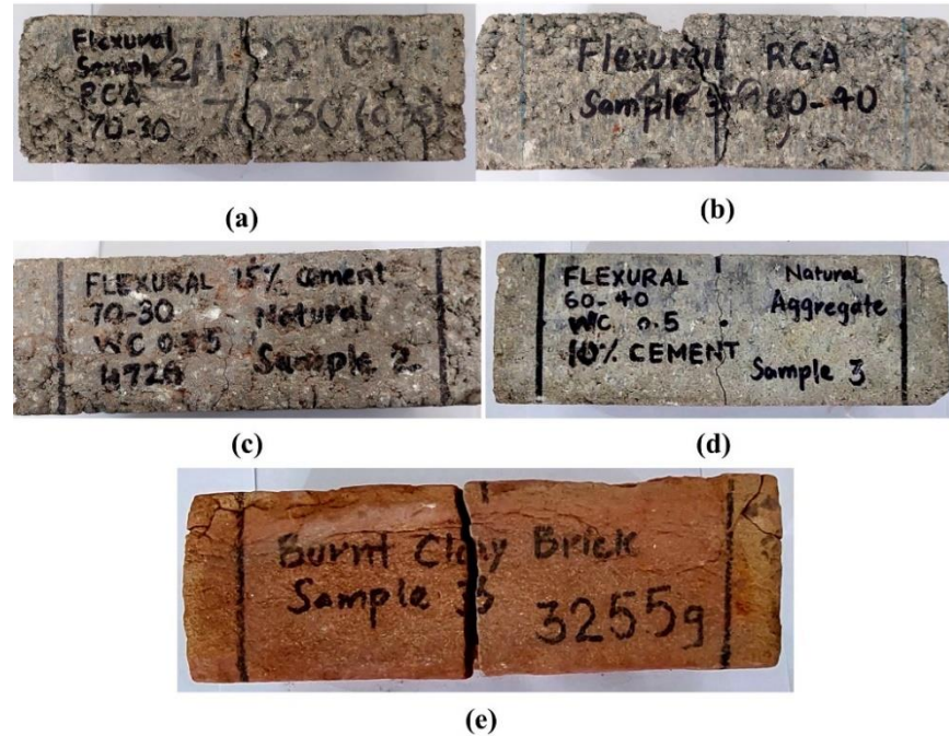
Figure 9. Failure modes of bricks under three-point bending test (a) RAC-70C30F brick (b) RAC-60C40F brick (c) NAC-70C30F brick (d) NAC-60C40F brick (e) Burnt clay brick.
